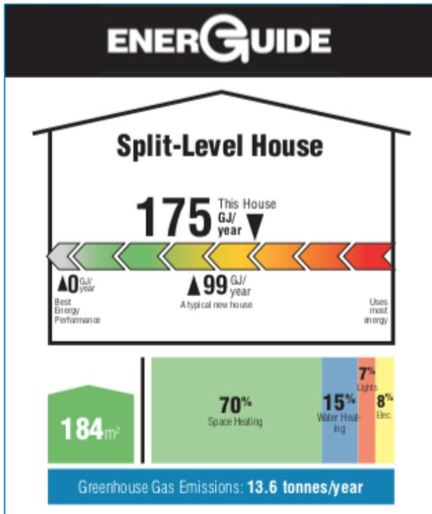
The Split-Level house was built in the 1970's, with RSI 2.1 in the walls and in the attic. At 184 m<sup>2</sup>, it is just below average in size.
