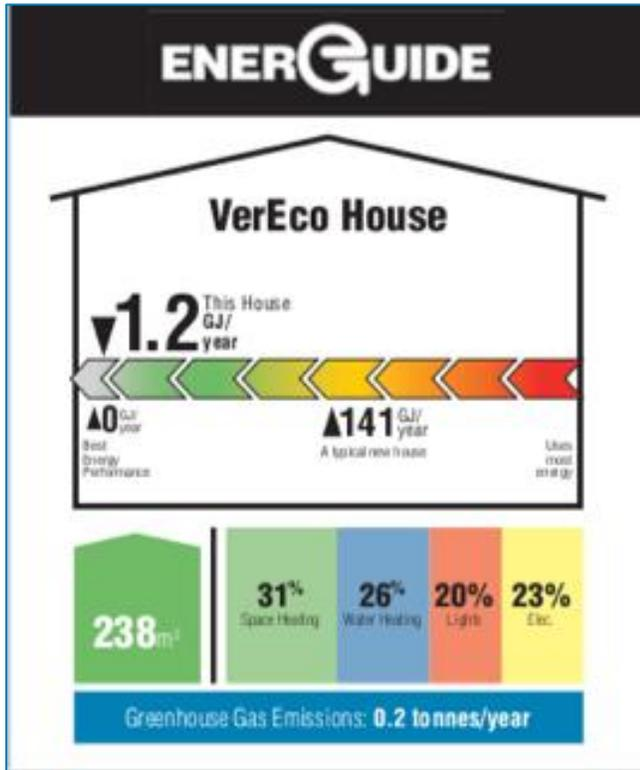
The Vereco house was built in 2010 but built to be very efficient with RSI 7.6 in the walls and RSI 14.1 in the attic. At 238 m<sup>2</sup>, it is above average in size. Designed to use 53GJ/year, it produces almost as much energy as it uses, from solar panels that provide electricity.
