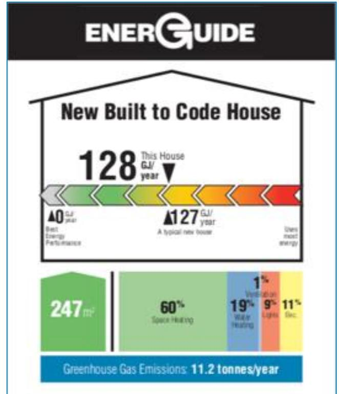
The New Built to Code house was built in 2019, with RSI 3.9 walls and RSI 8.8 in the attic. At 247 m<sup>2</sup>, it is above average in size.
