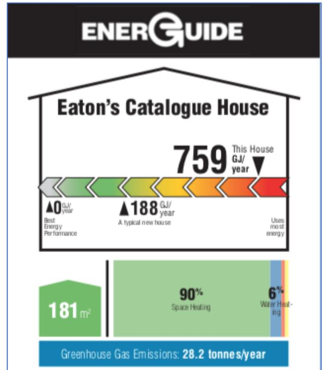
The Eaton's house was built in 1910, with no insulation in the walls or in the attic. The building materials provide RSI 0.7 for the walls and RSI 0.3 in the attic. At 181 m<sup>2</sup>, it is below average in size.
